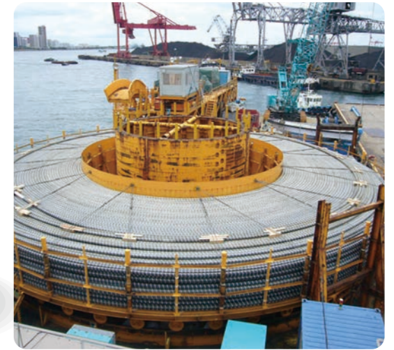
Cables being loaded for shipping
